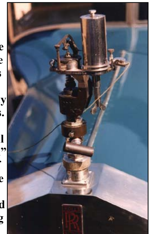
"I don't know what it does, but it does it magnificently". It is, in fact, a device for measuring the efficiency of steam engines.
